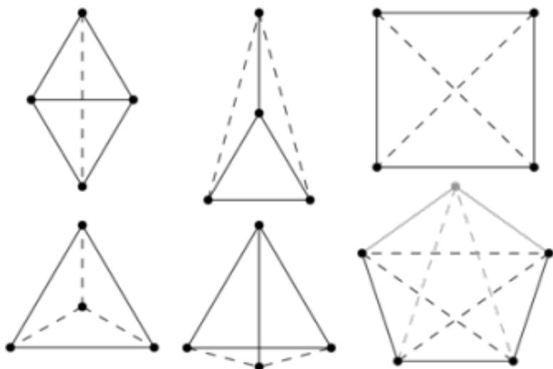
Short edges are represented by **straight lines** while long edges are represented by **dashed lines**. One of these solutions can be extended to 5 points that only use two distances, see bottom right picture.
