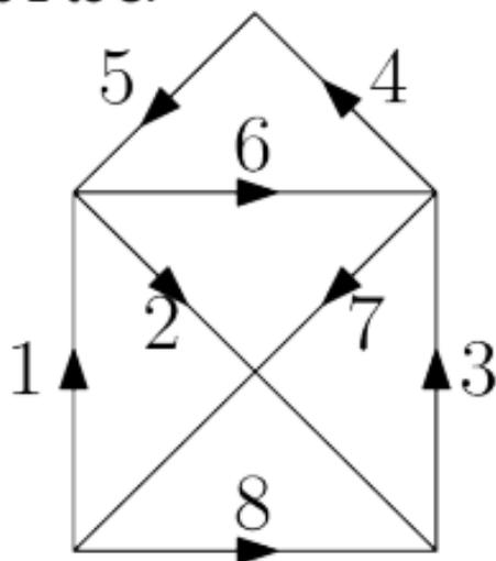
This kind of path is called an Euler path, and it is called an Euler circuit if it starts and ends in the same point. The degree of a vertex is the
